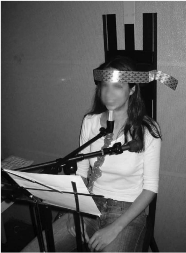
FIG. 3. Head and transducer stabilization setup. The speaker's head is encompassed by the moldable head stabilizer, which can be moved up and down on the Velcro strips against the wall of the soundproof booth. Another Velcro strap is pulled against the speaker's head for further stabilization. The transducer is stabilized with a microphone stand.
