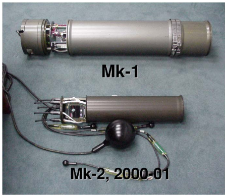
FIG. 5. Telesonar Testbed used to collect data.
